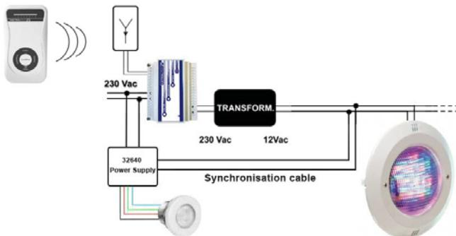
Diagram for LumiPlus Projectors PAR56; Jelly; Flat and Standard for Fountains with Mini and Micro
