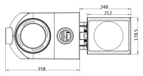
Figure 1: Overall product dimensions in mm
